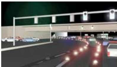
LRC rendering of proposed LED marking system for a complex intersection
